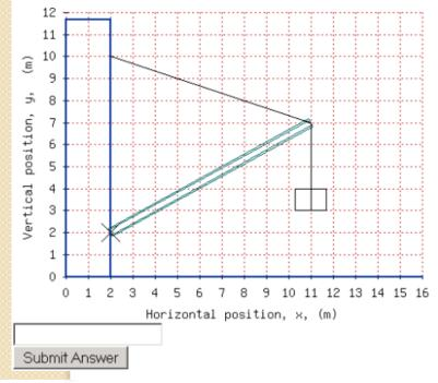
1 pt A crate with a mass of 177.5 kg is suspended from the end of a uniform boom with mass of 88.5 kg. The upper end of the boom is supported by a cable attached to the wall and the lower end by a pivot (marked X) on the same wall. Calculate the tension in the cable.
